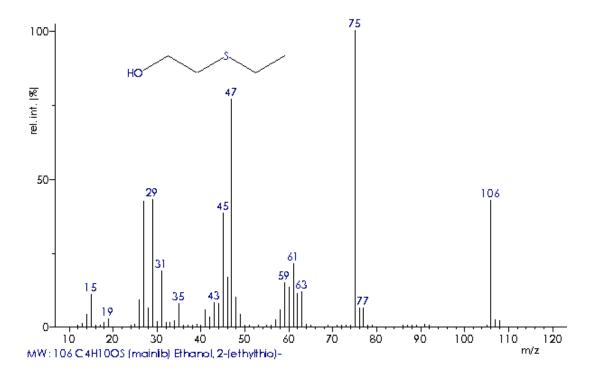
The (presumed) monoisotopic molecular ion peak is of medium intensity, located at m/z 106, and exhibits an isotopic pattern that cannot result from carbon alone, but Cl and Br can be excluded. In case of Si, the pattern wouldn't allow for additional carbons. Thus, S is reasonable.
