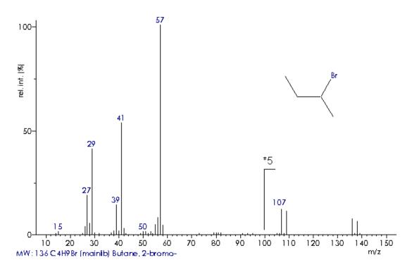
Starting from m/z 100, the intensities are shown magnified fivefold. Crawl across the mass spectrum to identify typical isotopic patterns, obvious mass differences, i.e., neutral losses, and/or well-known fragment ions or fragment ion series:
